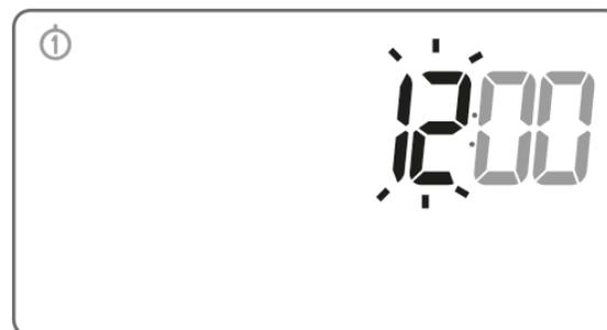
Turn the knob to the left or right to set the correct value on the minute segment and confirm using the **OK** button.
