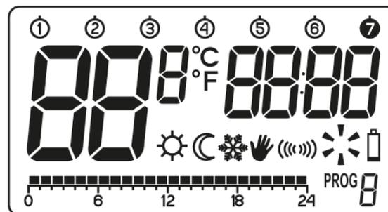
After a while, AURATON Libra will automatically switch to the time setting mode. A flashing item on the screen means that the device is currently in the edit mode. Turn the knob to the left or right to set the required hour and confirm using the **OK** button.
