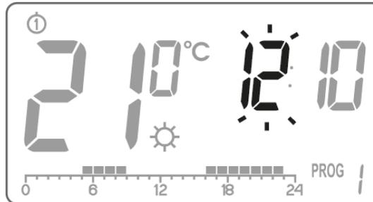
2. Turn the knob to the left or right to set the required hour and confirm with using the
