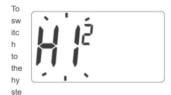
resis change mode, hold down the ♥, ▲ and <sup>©</sup> buttons simultaneously for 3 seconds. The hysteresis change mode is signaled by the **HI** inscription . Use the ♥, ▲ buttons to change the hysteresis settings.
